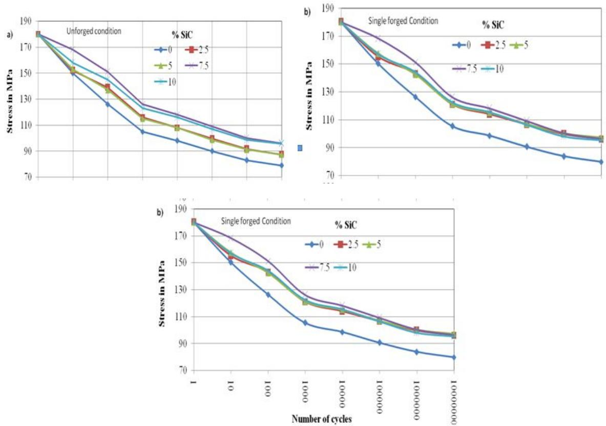
**Figure 2: Wöhler curves for Al and Al/SiC MMCs for
