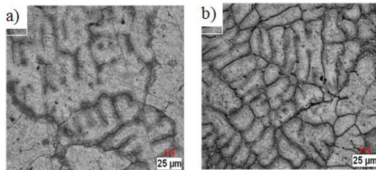
**Figure 1: The Optical Micrograph of the Al/10 % Sic MMCs A) As Cast
