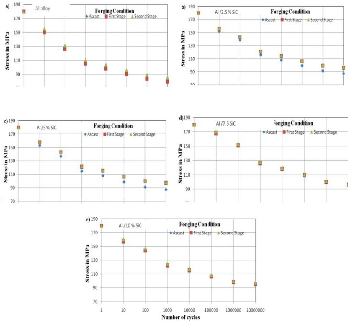
**Figure 3: Wöhler Curves for Ascast, First Stage Forging and Second Stage Forging For Al, Al/ 2.5%, Al/5%, Al/7.5% And Al/10% Basalt Short**
