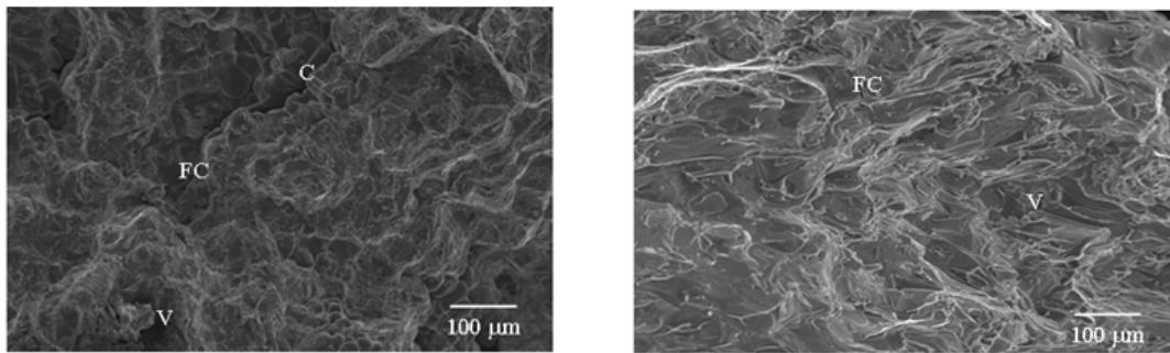
**Figure 5: Fracture Surface of a) un-Forged and b) Forged Condition Al 7075/5 wt % of Basalt Short Fiber MMC S after Fatigue Test. C-Main Crack, V-Void in Matrix Alloy Fracture Studies**
