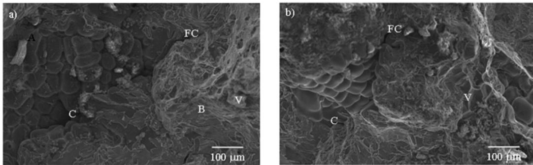
**Figure 4: Fracture Surface of a) un-Forged and b) Forged Vondition Al7075 Allay Specimen After Fatigue C- Main Crask, Fc- Fatigue Crack, V-Void In Matrix Alloy**
